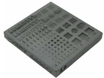
Dimensional Bar for finishing tests – before and after NAM cleaning process
