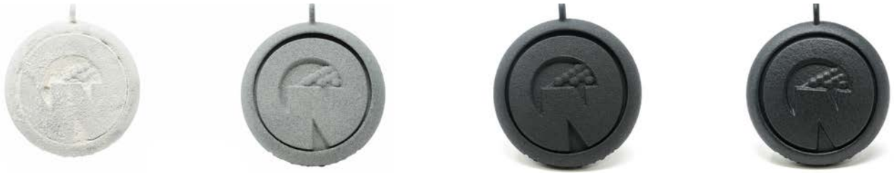
HP PA12: raw – NAM Cleaning – dyeing – NAM Finishing
