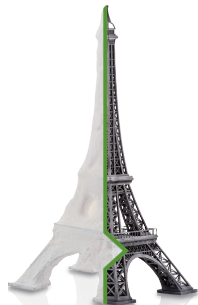
MJF printed Eiffel Tower before and after NAM cleaning process
